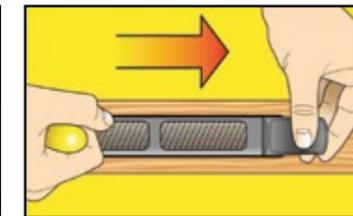
For **SMOOTHING** and **FINISHING**, use the tool parallel to the direction of the cut
