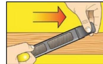
For **FAST CUTTING**, use the tool at an angle of about 30° in the direction of the cut
