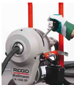
Engage clutch, cable spins
