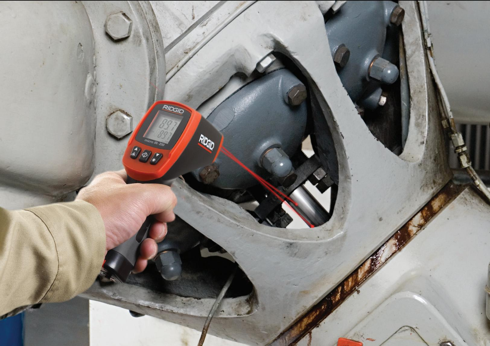
The RIDGID® micro IR-200 Non-Contact Infrared Thermometer provides simple, quick and accurate surface temperature readings at the push of a button. Simply squeeze the trigger and point the ultra-sharp dual class II lasers at the surface being measured.
