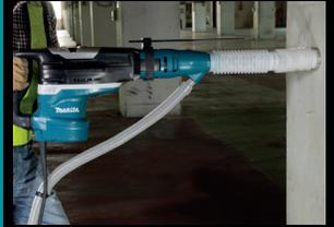
Helps reduce dust created from concrete drilling
